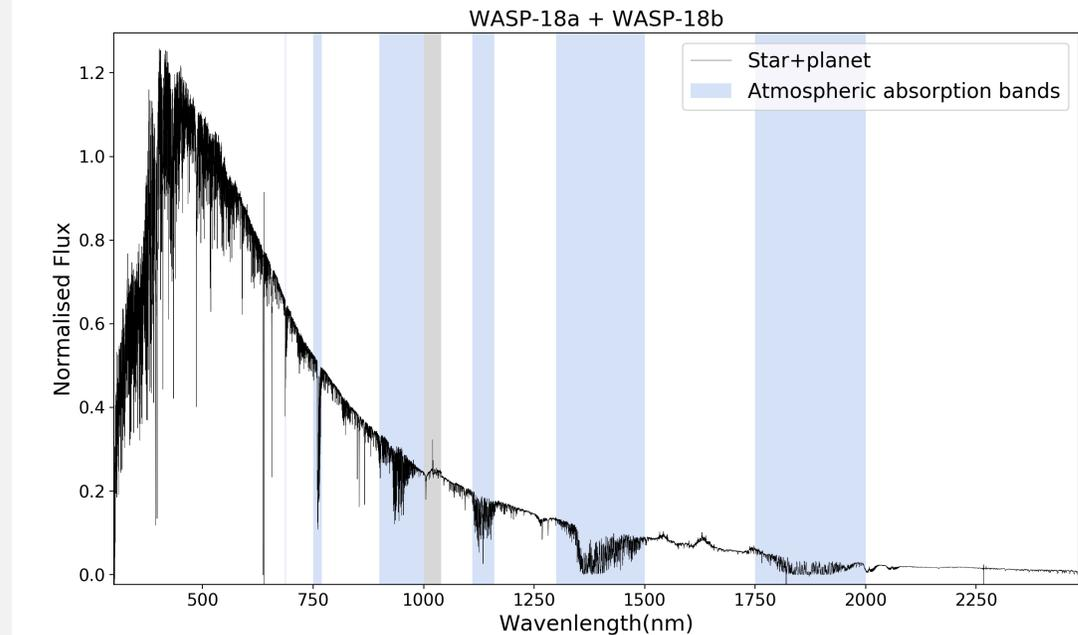
**Fig. 3** - The UV, visible and infrared (IR) arms are combined to produce a full spectrum of the WASP-18 system while the planet is in its out-of-eclipse phase. The grey shaded area represents the transition between the visible and IR arms, which is excluded from further analysis because of its poor calibration level. Atmospheric absorption bands also interfere with the planetary signatures hence we will not consider them.
